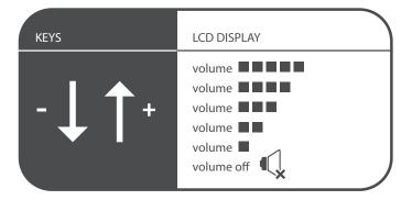
The new volume level is shown on the display for 2s then saved.
