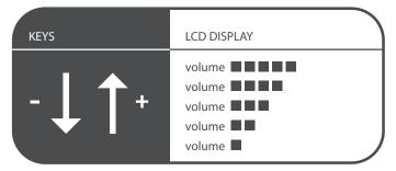
The new volume level is shown on the display for 2 seconds then saved.
